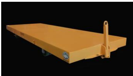
40,000 lb. capacity caster steer trailer as it leaves our facility
