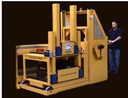
**Titan** Carts are ergonomically designed to reduce operator fatigue and deck surface or mechanical push/pull system options allow for the safe and easy transfer of molds and dies to press or rack.
