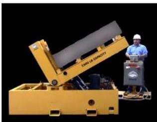
**Titan** Coil Upenders or Coil Tippers allow the user to load palletized metal coils onto the deck, then invert them to the horizontal orientation for feed line loading, to provide safe and efficient delivery of coils throughout the manufacturing facility.
