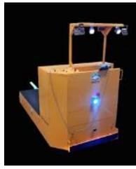
(LEFT) **Titan** Free Range Transporters, with capacities up to 160,000 lbs., are offered with a variety of safety options including: wireless remote control, laser scanner collision avoidance system, blue/red light pedestrian warning, custom color paint, audible alarms and strobe, E-stop bumpers, collision avoidance sensors, access steps and hand rails, head and rear lights, rear view mirrors, and safety gates/chains at on-board operator station.
